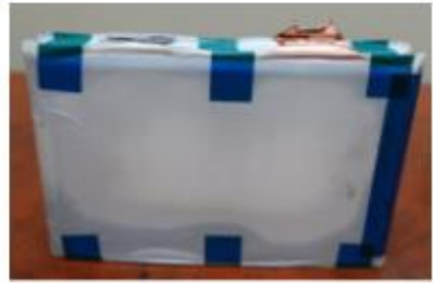
100 Ah cell prismatic stacking
